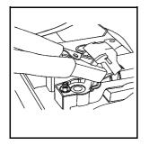
Connect the red positive (+) cable to the positive (+) terminal of the vehicle with the dead battery. Use a remote positive (+) terminal if the vehicle has one.
